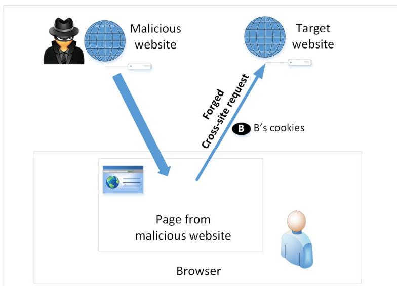
Figure 10.2: How a CSRF attack works
